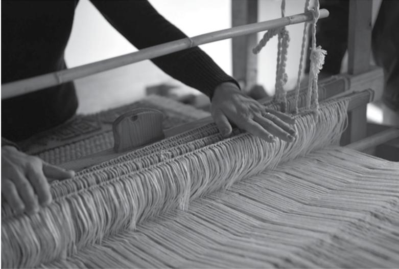
Figure 1. The Almalaguês looms have remained unchanged over centuries, incorporating a minimum number of metal parts in a largely wooden construction.
